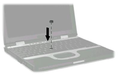
Replacing the pointing stick cap
